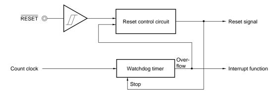
Figure 8-1. Block Diagram of Reset Function
