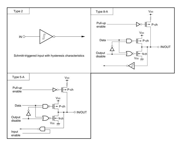
Figure 3-1. Pin Input/Output Circuits
