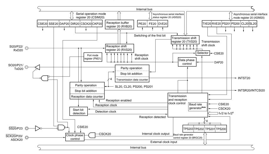
Note See Figure 5-19 for the configuration of the baud rate generator.
