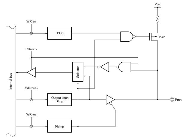
Caution Figure 5-2 shows the basic configuration of ports 0, 1 and 3. This configuration varies depending on the alternate pin functions.
